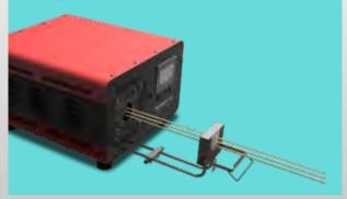
Calibrate alumina laboratory standard & industrial thermocouples
