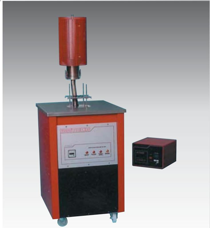
temperature stability and uniformity cannot be achieved in the fluidized medium itself. They are obtained by using large metal blocks or by inhibiting the fluidizing action in the powder around the work piece - either locally, or by completely collapsing the bed at the required temperature, this is not the case with the 875. A full evaluation report is available upon request. The bath is fully commissioned, tested and charged with the correct amount of aluminium oxide powder before despatch.
