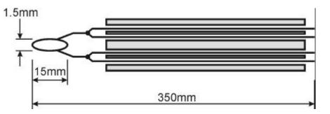
The type R T/Cs had exposed junctions and were each housed in 4mm diameter 2 bore ceramic tube. They were referenced using an Isotech Zeref 136/6 and their outputs were measured using a Solartron 7075 digital multimeter.
