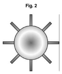
Isotech term this 'the spider'. Spiders can be made to the customer's requirements including having a tube which passes through the ball so that T/Cs with multiple junctions along their length -as used in the semiconductor industry- can be calibrated.
